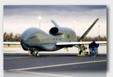
caused electrical damage inside the LRU, which cut power to the actuators that controlled the unmanned aircraft's ailerons and spoilers. Within 1min of the power failure, the aircraft lost control after hitting minor turbulence.
